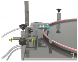
**4.** Assembly of the jar guide rod: Fig. 5
